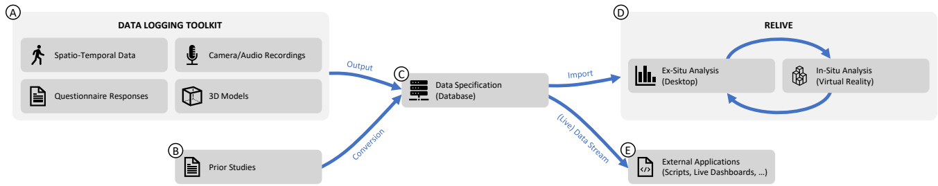
Figure 5: Logging and evaluation overview. This environment supports researchers throughout the all stages of a study: (A) An open data logging toolkit can facilitate data capturing, including spatiotemporal data (e.g., movement data from AR HMD), video data (e.g., imported or automatically captured from network cameras), questionnaire responses, and 3D models. (B) Data from prior studies can be converted to the data specification for use within RELIVE. (C) Our data specification contains holistic data about a study, and can be easily accessed by external applications. (D) RELIVE uses the data specification to enable a holistic study data analysis and reconstruct the original study setting. (E) Data from an ongoing study can be streamed to (and parsed by) external applications, enabling an analysis using bespoke scripts or live dashboards.
