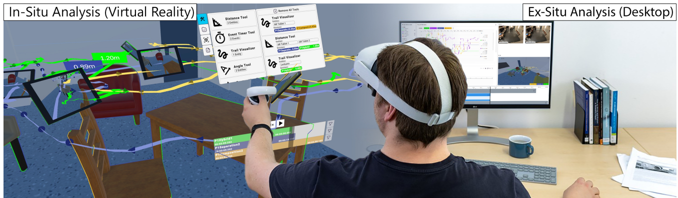
Figure 1: The RELIVE mixed-immersion tool. RELIVE combines an immersive analytics virtual reality view (left) with a synchronized non-immersive visual analytics desktop view (right) for analyzing mixed reality studies. The virtual reality view allows users to relive and analyze prior studies in-situ, while the desktop facilitates an ex-situ analysis of aggregated data.
