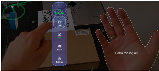
Figure 2: Screenshot of the mode selection interface. The menu is active when the palm of either hand is facing up. The menu can be interacted with using the opposite hand.
