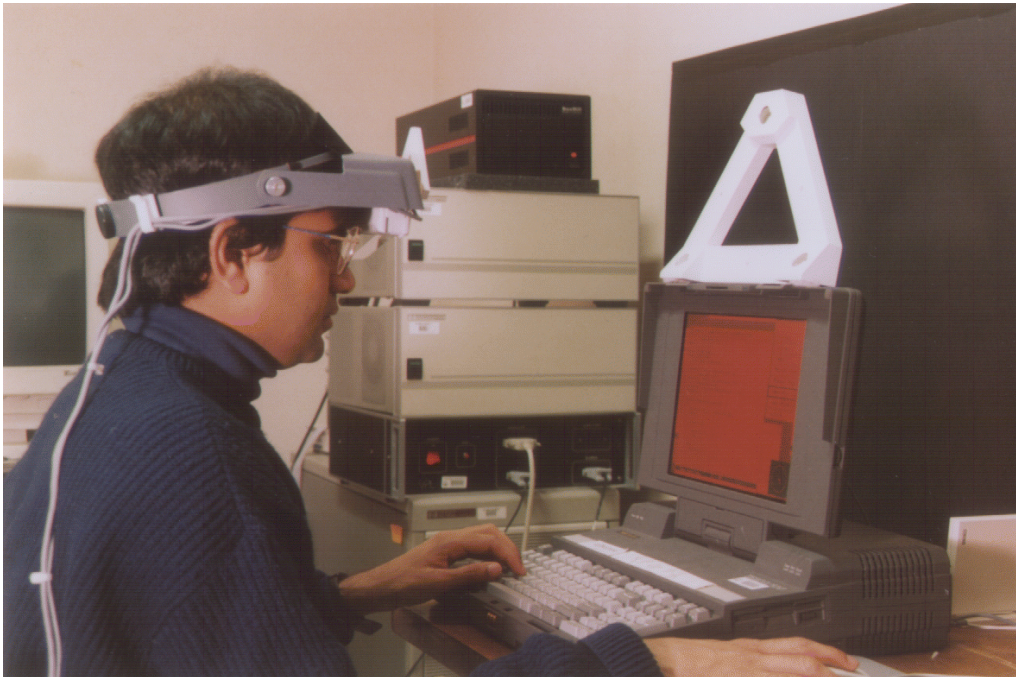
Figure 2.4: The setup of Feiner and Shamash [97]. A Hybrid User Interface combining a head-worn device for augmented reality and a laptop.
