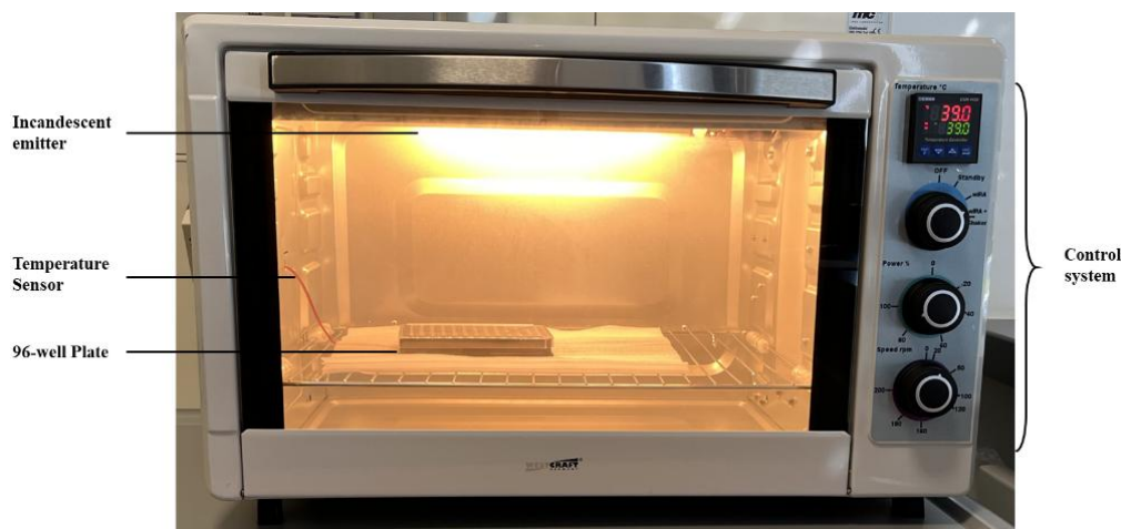
Figure 16: Placement of the treatment plate in the IRAcubator heat treatment device
