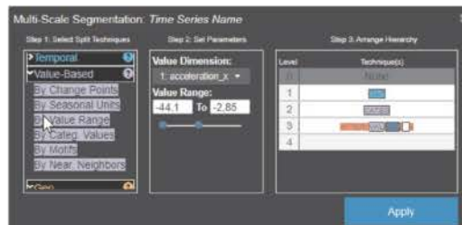
Fig. 6. The query building dialog is shaped by three steps: choose a segmentation technique, set parameters, arrange the technique/hierarchy.
