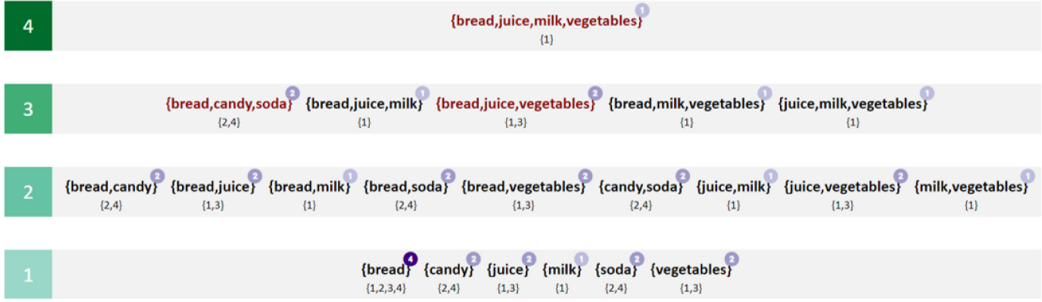
Fig. 3. The search space of an itemset mining algorithm visualized as a Hasse diagram [72]. The length (i.e., cardinality) is encoded in the vertical position. The support is denoted in purple. The red itemsets occur in the input data.
