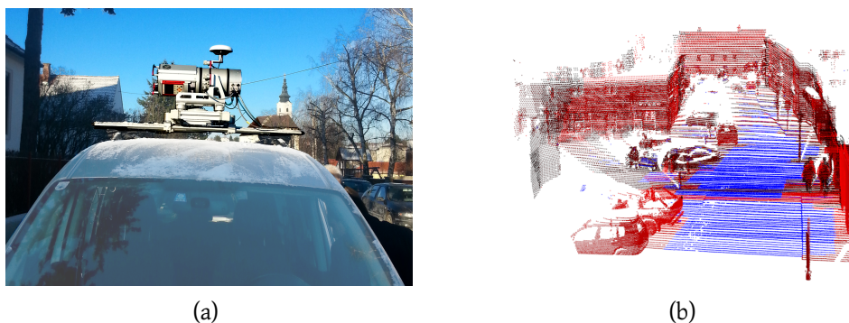
Figure 3.10: (a) Sensor mounted on the roof of a car. (b) Classified accumulated point cloud. Non-classified points are color-coded from black to red. The color depicts the timestamp when a point is recorded, black points are the oldest while red points are the newest. Blue points are classified as ground.
