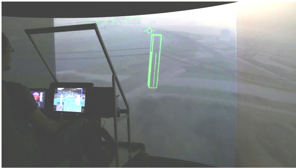
Figure B.2: Box meshing with additional distance cue on a HMD in simulator environment: Objects far away are faded out and replaced by a symbol representing the principal components of the cluster in a simulated DVE scene.
