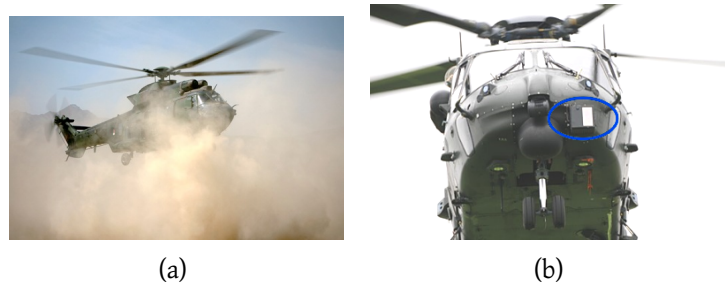
Figure 1.1: (a) Helicopter in a DVE situation during a brownout [DDP]. (b) The LiDAR sensor is highlighted in a blue ellipse mounted in front of a NH90 helicopter [Air].
