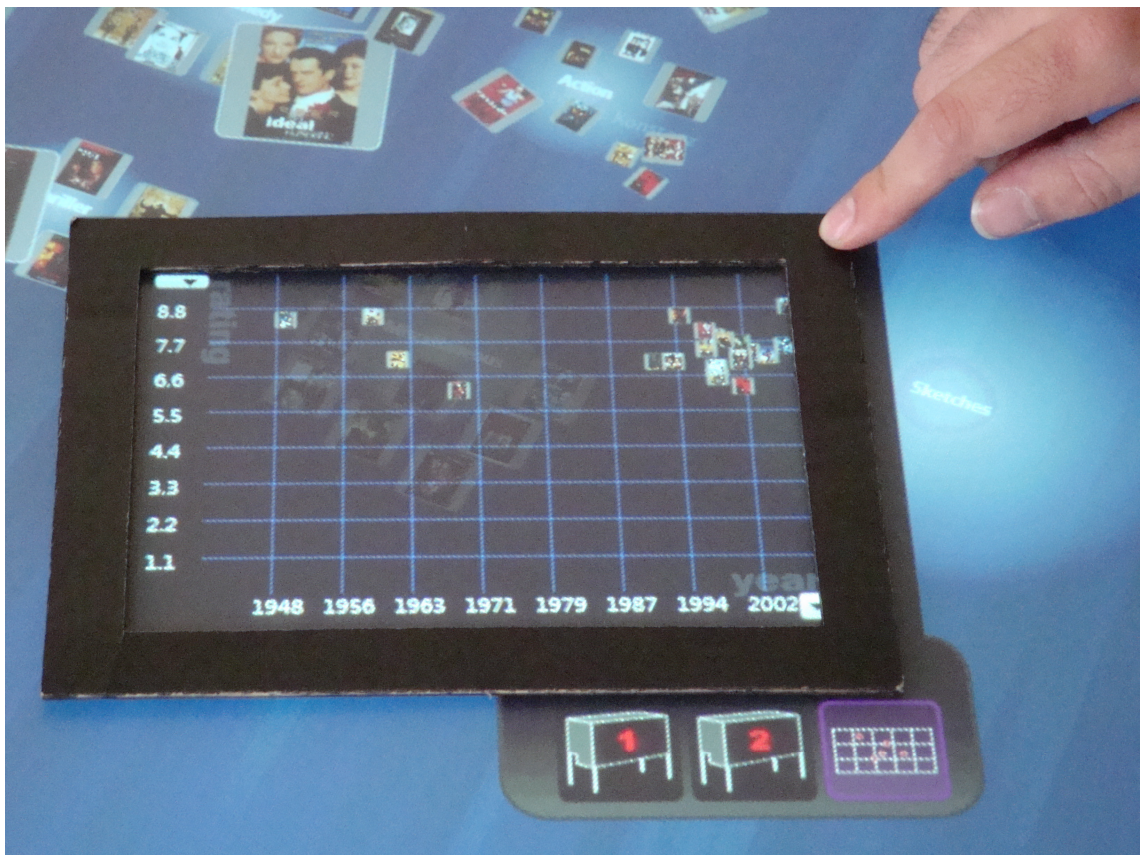
Figure 17 – A tangible lens object can be used to view the underlying objects in a scatter plot. In this case, year on the x-axis and user rating on the y-axis.
