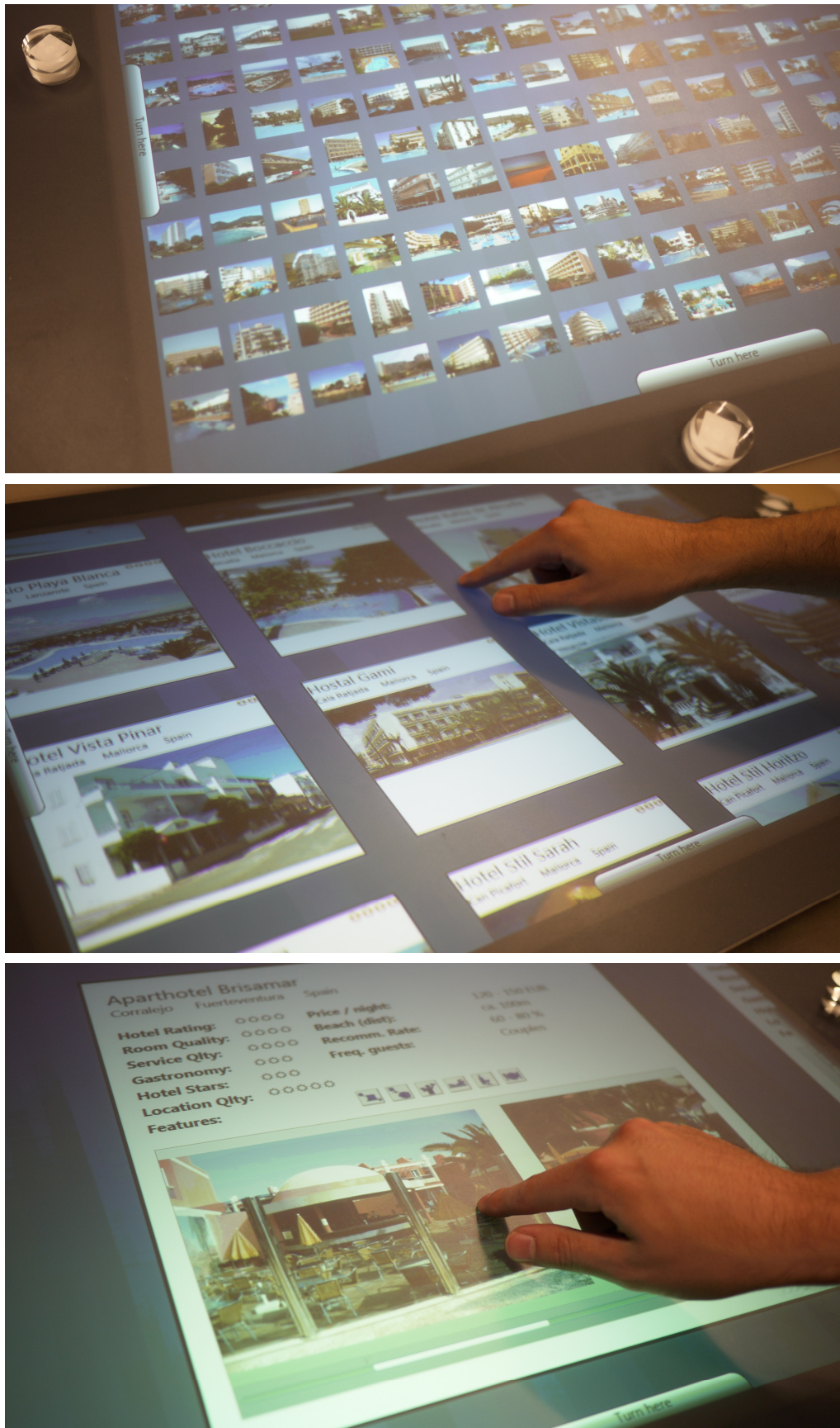
Figure 36 – The grid structure on the tabletop with the content of the catalog. Details and user-generated content can be accessed by zooming in. Source: (Jetter, Gerken, Zöllner et al. 2011).
