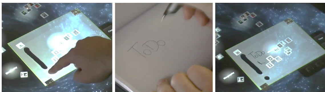
Figure 93 – A transparent frame with markers serves as Post-It lens . Left: Touch writing. Middle: Handwriting with Anoto digital pen & paper. Right: Ink strokes immediately appear on virtual Post-It.
