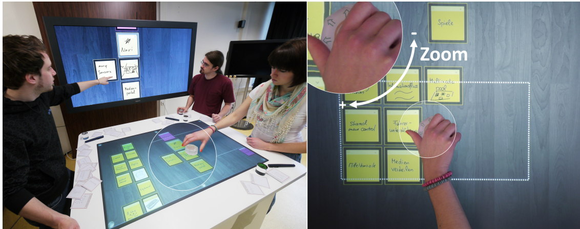
Figure 94 – The AffinityTable setup (left). By sliding and rotating the camera token on the overview-tabletop users can control the content of the vertical high-resolution 4K display.
