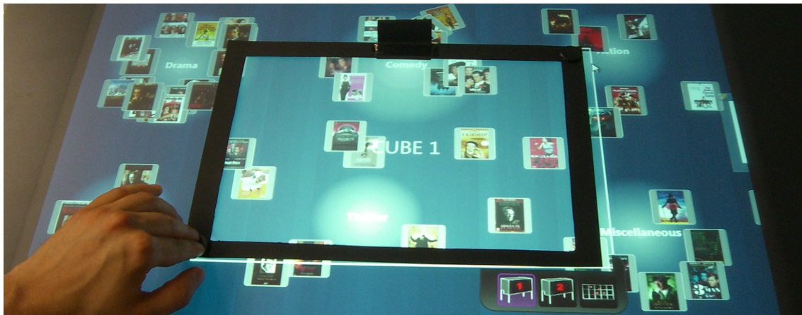
Figure 91 – A ZOIL-based prototype with a passive tangible lens on a Microsoft Surface tabletop. The mode of the lens can be selected with the virtual buttons in the lower right corner of the lens.
