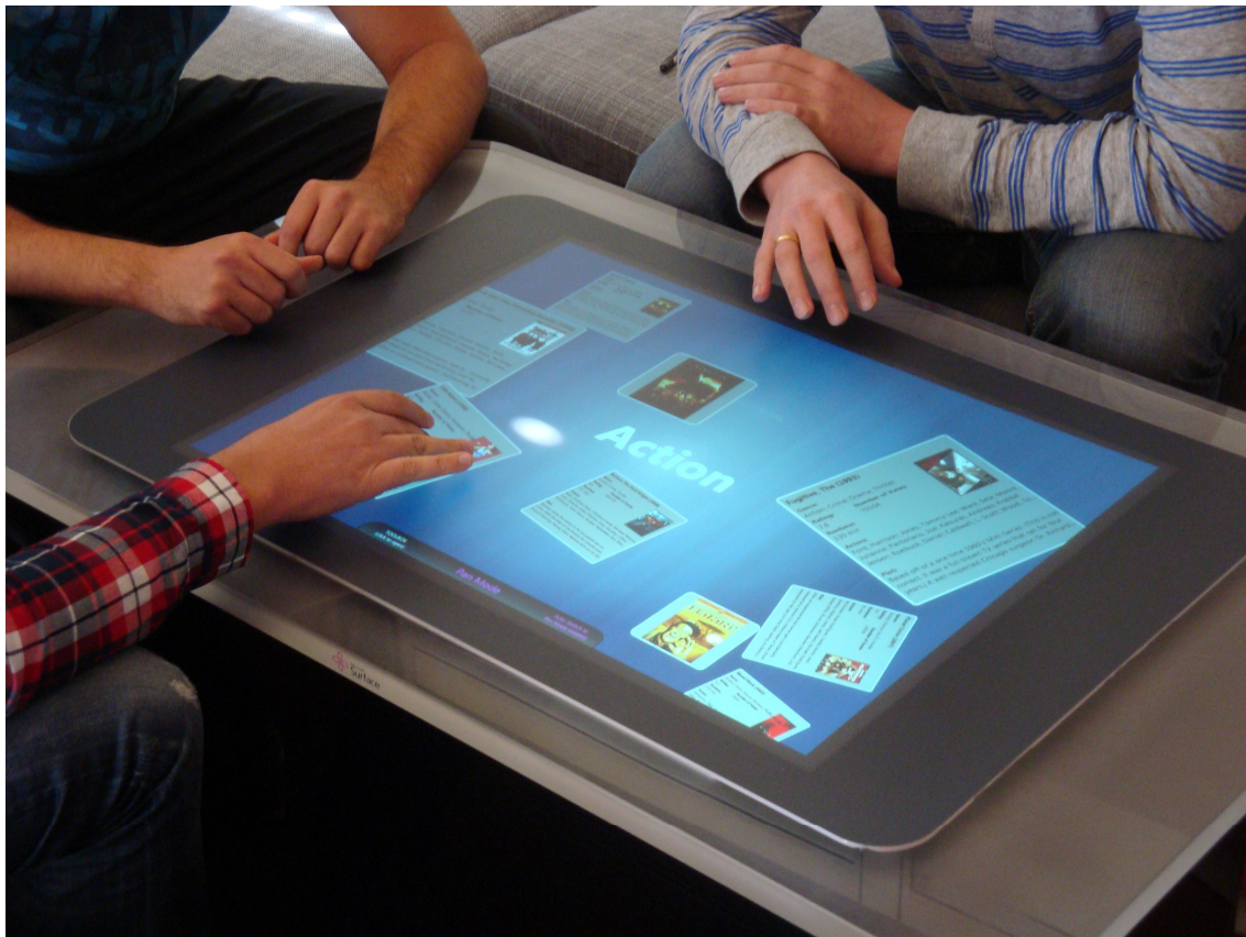
Figure 13 – A tabletop computer can be used to collaboratively explore and rearrange the movie objects in ZOIL’s zoomable information landscape.
