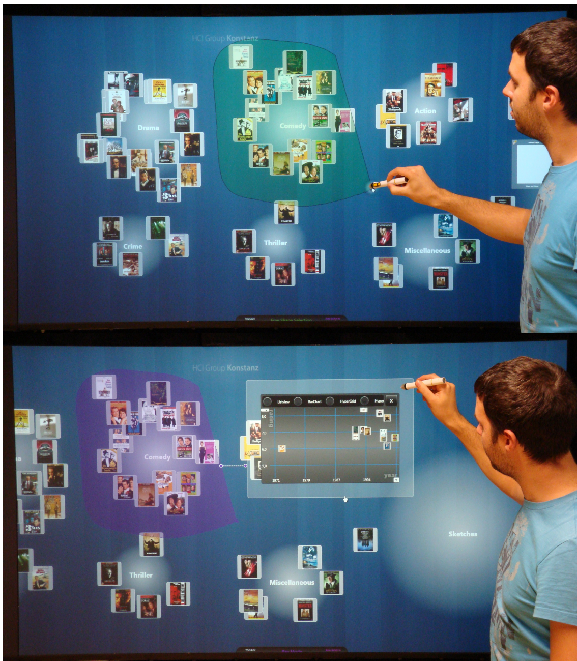
Figure 18 – Pen input on a vertical display can be used to draw a shape for selecting objects (top) and displaying a visualization of the contained objects (bottom).
