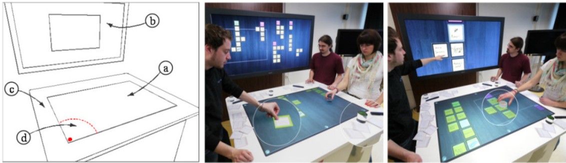
Figure 60 – The AffinityTable consists of a tabletop as shared action space (a) and a vertical 4K high-resolution display as shared reflection space (b). Source: (Geyer, Pfeil, Höchtel et al. 2011).
