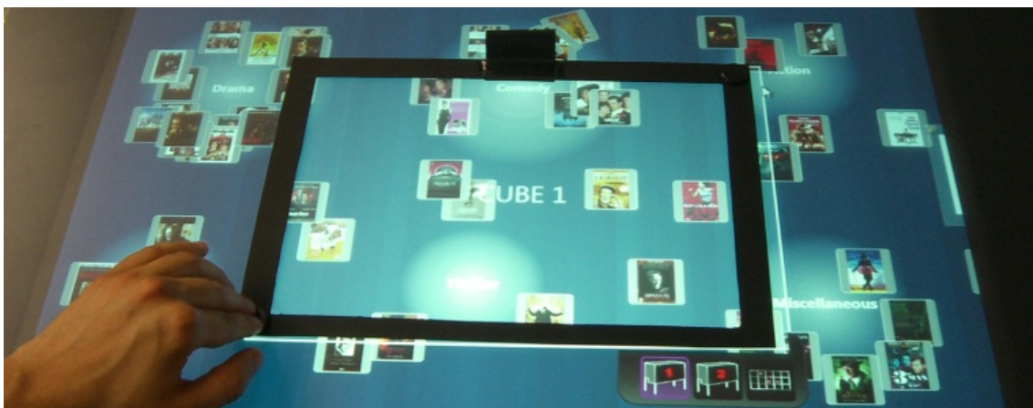
Figure 16 – The physical camera lens object on the tabletop can be used to establish coupling between the content that lies within the boundaries of the lens and the remote vertical displays.
