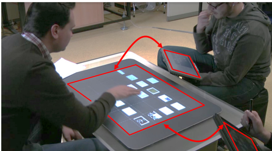
Figure 27 – DeskPiles running on a tabletop and two tablet PCs. They are connected to the same meeting server to provide a shared information landscape on all devices.
