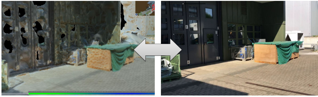
Figure 2: The left image shows a static mesh of the reconstructed scene. The right side shows the original video frame. The analyst is able to seamlessly switch between the reconstructed scene and the imaging material.
