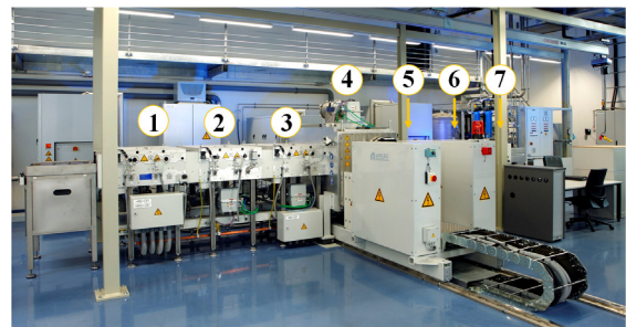
Figure 1: ATON 500 inline high-rate evaporation system installed at the ISFH. The modules indicated by numbers in the photo above will be explained in the schematic drawing in Figure 2.
