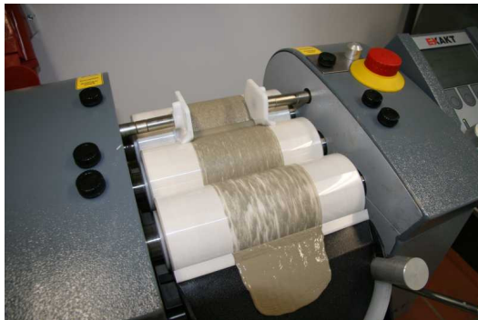
Figure 2: Three roll mill on which an ink is homogenized by successively reducing the distance between the single rolls.
