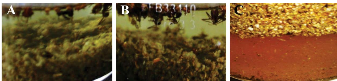
Fig. 51: Comparison of solvents to separate bodies of dead ants and waste particles. A: Hexane; B: Methanol; C: Water.
