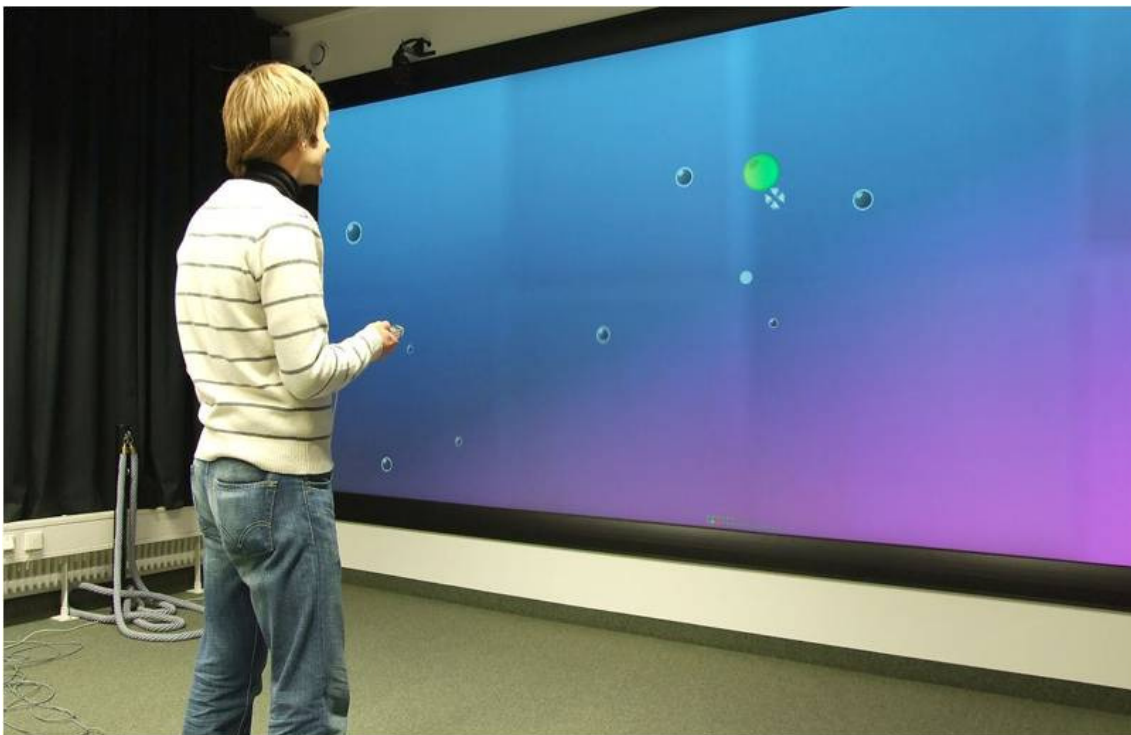
Figure 6: Study Setup: Multi-directional tapping task (green bubble represents target object)
