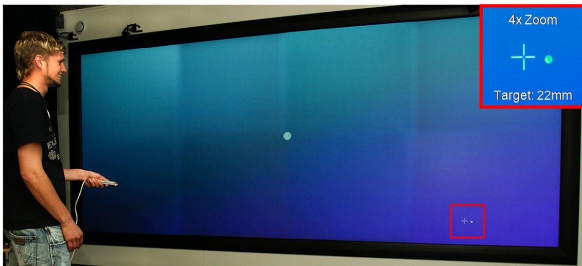
Figure 50: The Adaptive Pointing technique in combination with a laser-pointer as input device in front of a Powerwall
