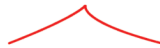
Fig. 7. A cubic Bézier curve with a “kink”, i. e. a point of large curvature, near the middle. The curve is C^1 smooth; but the kink, together with the limits of human perception and screen resolution, mean that the curve does not look smooth.
