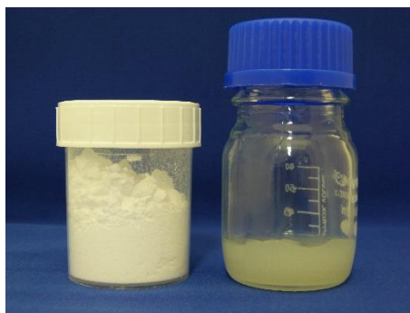
Figure 7.3: Comparison of a moderately branched polyethylene ( left , 6,300 \text{ g mol}^{-1} , 50 branches / 1,000 C) and a highly branched ethylene oligomer ( right , 1,700 \text{ g mol}^{-1} , 80 branches / 1,000 C).
