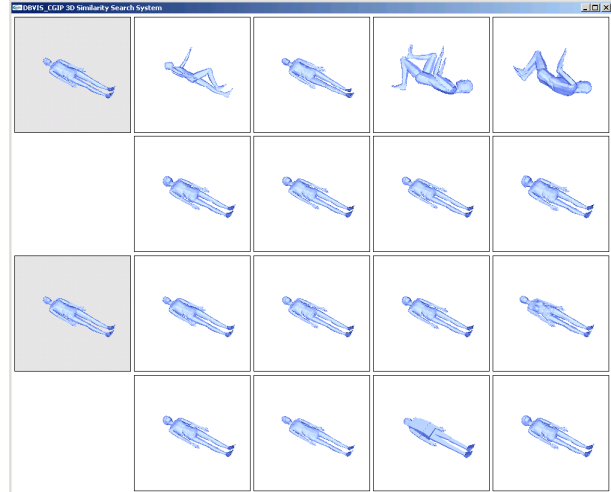
Figure 5. Example query in the humans class. The first query was conducted using the shape spectrum method and retrieves different articulations of the same model on the first ranks. The second query was conducted using the depth buffer method, and retrieves human models having the same articulation as the query object.
