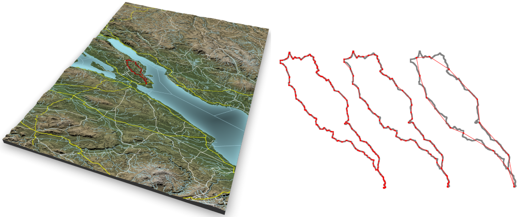
■ Figure 1 Left: 3D map (created with rayshader [18]), overlaid with linear features extracted from OSM, namely waterways (blue), primary and secondary roads (yellow and white), and a GPS track (red). The waterways and roads consist of roughly 240,000 points in total, the GPS track of 1481 points. Right: Simplifications of the GPS track with 10%, 5% and 1% of the original points in red (original track for visual comparison in gray).
