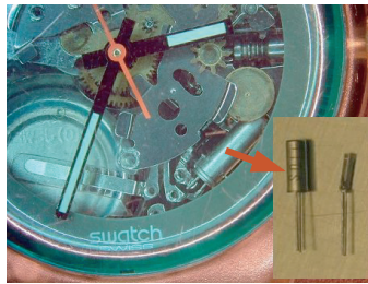
Figure 4.3: Watch crystal (based on a figure from [120]). The insert shows a photo of both of the tuning forks within the can and removed from the can.
