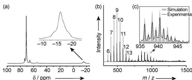
**Figure 2.** a) Solid-state  $^{13}\text{C}$  NMR spectrum and b) MALDI-TOF mass spectrum of the  $[\text{MeZnOPEG}_{400}]$  gel; c) comparison of the isotope pattern correlating to one of the high-mass signals of the dimeric  $[\text{MeZn}_2(\text{OPEG})_2]$  cluster.
