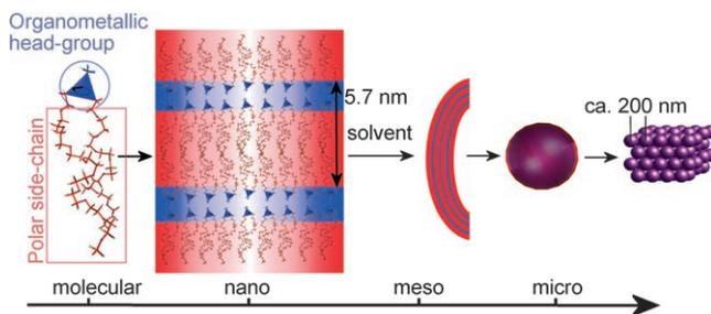
**Figure 5.** Mechanism of hierarchical self-organization for the  $[\text{MeZnOPEG}_n]$  materials starting with dimers at the molecular scale (image on the far left), which assemble into lamellar structures. In contact with toluene, curvature is enforced which leads to large spherical aggregates that finally pack into microscopic domains (image on the far right).
