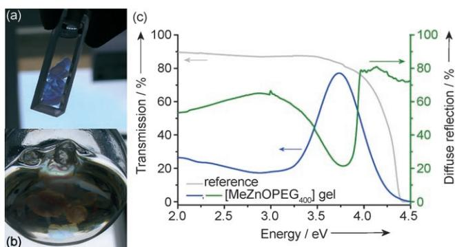
**Figure 1.** Optical properties of the  $[\text{MeZnOPEG}_n]$  gels ( $n = 400$ ). a) Photographic image of the material in transmission mode, b) photographic image of the gel from a different angle, and c) UV/Vis spectra.
