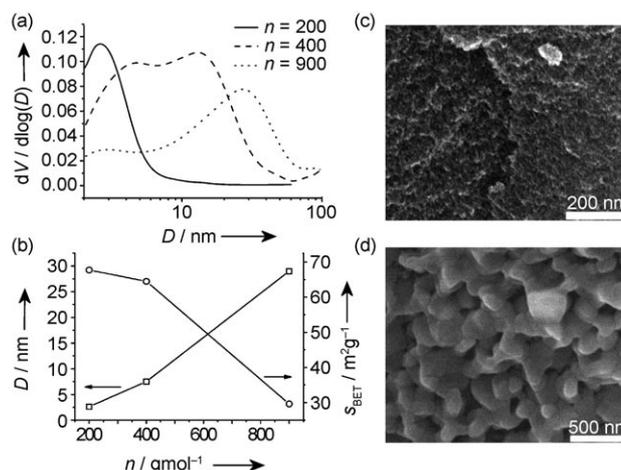
**Figure 7.** a) Barrett–Joyner–Halenda (BJH) pore-size distributions from  $\text{N}_2$ -physorption measurements (see Supporting Information) for three zinc oxide materials obtained from  $[\text{MeZnOPEG}_n]$  with different PEG chain lengths. b) Correlation between PEG chain length, pore size, and BET surface area ( $S_{\text{BET}}$ ) for the prepared materials. c, d) SEM images recorded at different magnifications for ZnO prepared from  $[\text{MeZnOPEG}_{400}]$ .
