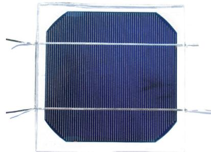
**Figure 1:** Photograph of a homogenous emitter solar cell embedded in Silicone A
