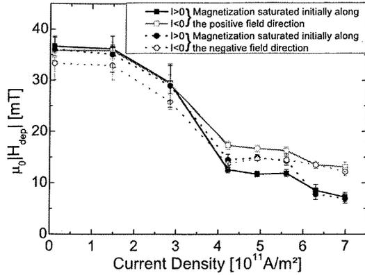
FIG. 2. (Color online)  $|H_{\text{dep}}|$  as a function of the injected current density for a constant cryostat temperature  $T_{\text{Cryo}}=100$  K and for both initial magnetization configurations. The measurement points represent the mean values of  $|H_{\text{dep}}|$  averaged over at least eight repetitions, while the error bars show the standard deviation.
