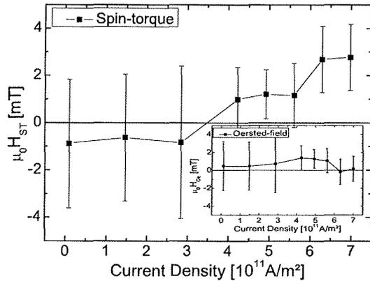
FIG. 3. The deduced contributions for spin torque and for Oersted field (inset). The efficiency  $\epsilon$  is deduced from a linear fit through the origin (zero spin torque for zero current density) using the points with the lowest Oersted field contribution.
