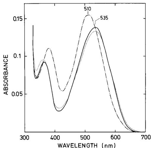
Fig. 4. Comparison of the absorption spectra of free and luciferase-bound 1-d-FMN, along with that for the protonated form of 1-d-FMN. Cuvettes contained 20  $\mu$ M 1-d-FMN with or without luciferase (40  $\mu$ M) in 0.01 M phosphate buffer, pH 7.0, at 4°C. Protonated 1-d-FMN (same concentration) at  $H_0 = -1$ , measured at 20°C. (—) Free 1-d-FMN; (----) luciferase-bound 1-d-FMN; (- - -) protonated form of 1-d-FMN
