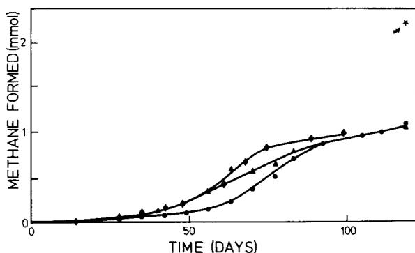
Fig. 2. Formation of methane from squalene by enrichment cultures. Experimental conditions were the same as described for Fig. 1. 50  $\mu\text{l}$  (105  $\mu\text{mol}$ ) of squalene was added as substrate. ◆, Enrichment culture Gö Sq from sewage sludge transferred 5 times; ●, same enrichment, transferred 7 times; ▲, enrichment culture Wo Sq from creek sediment transferred 7 times. Arrow points to the amount of methane calculated for complete methanogenic degradation.
