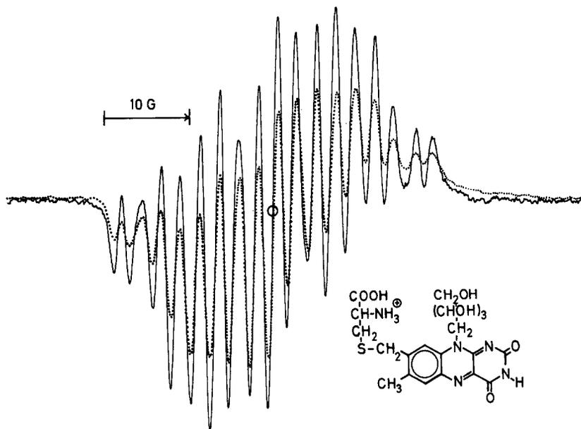
Fig. 5. Comparison of the ESR hyperfine structure of synthetical (—) and natural (- - -) MAO-flavin (IIb) [3] radical cations in 6 N HCl, reduced with  $\text{TiCl}_3$ , measured with a Varian E 3 at room temperature, 8 mW power and with a modulation amplitude of 1.0 G.
