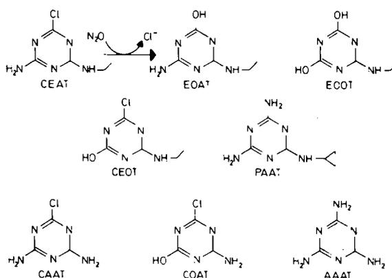
Fig. 1. The dechlorination reaction and *s*-triazines mentioned in the text. *s*-Triazines are abbreviated in the system proposed by Cook [11]: A, amino; C, chloro; E, ethylamino; I, isopropylamino; O, hydroxy; P, cyclopropylamino; T, *s*-triazine ring.
