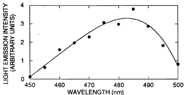
Figure 2. Bioluminescence emission spectrum with reduced 4H-FMN as the substrate. 4H-FMN in 0.5 mL 350 mM potassium phosphate, pH 7 was reduced with a dithionite solution in the presence of luciferase. Light emission was initiated by injection of 1 mL of a 0.01% decanal suspension in the same buffer and measured with a Perkin Elmer MPF-4
