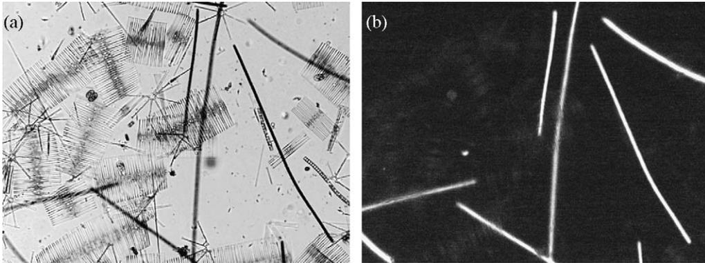
Fig. 3. (a) Light microscopy of a Lake Ammersee seston sample containing diatoms, other eukaryotic algae and cyanobacteria predominantly filamentous *P. rubescens* and (b) differentiation of cyanobacteria in the same field-of-view from eukaryotic algae using epifluorescence microscopy (magnification  $\times 100$ ).
