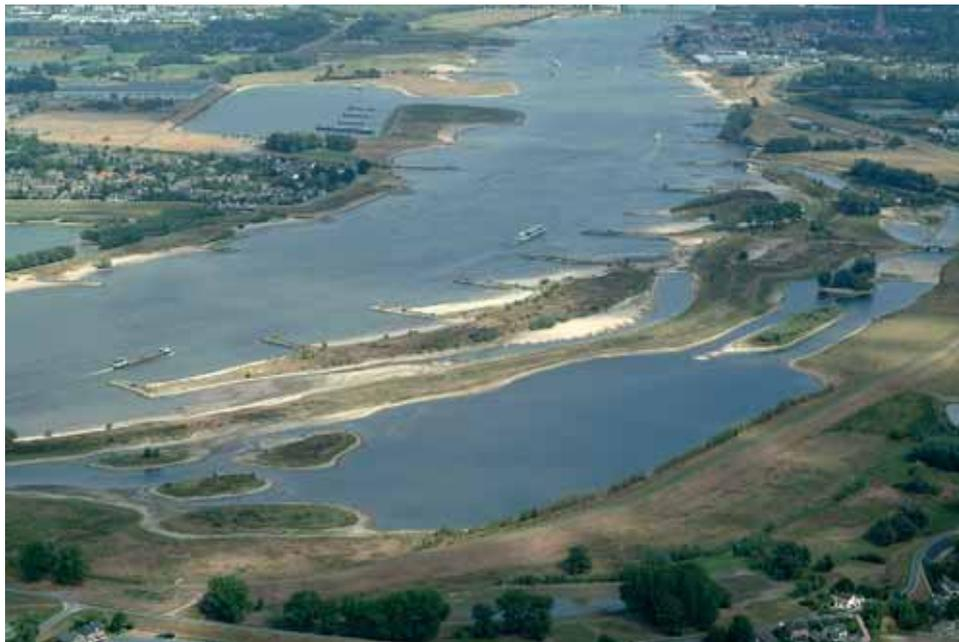
**PHOTO 6.12** Delta Rhine. Meander of the river Waal west of Zaltbommel in the Netherlands (river 933.5–938 km). The secondary channel (foreground) constructed in the forelands mitigates the effects of river engineering. (Photo B. Boekhoven, Rijkswaterstaat, The Netherlands).
