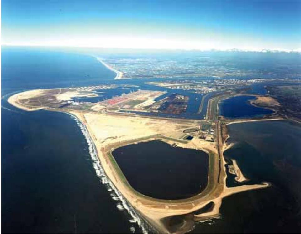
**PHOTO 6.13** Delta Rhine. Outflow of the Nieuwe Waterweg in the North Sea (top) with the heavily industrialized Maasvlakte and in the south (foreground) the large disposal site 'Slufter' for controlled storage of polluted river sediments. (Photo B. Boekhoven, Rijkswaterstaat, The Netherlands).
