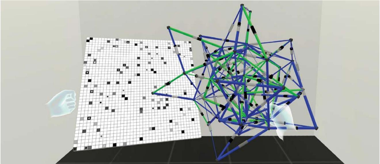
Fig. 1: A matrix representation (left) and a node-link diagram representation (right), both supporting the simultaneous visual comparison of two weighted networks in an immersive environment.
