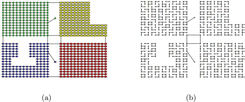
**Fig. 3.** In 3(a) the clustering determined by GMC for a grid-like graph is shown. The clusters are shown by the different shapes of vertices. In contrast, 3(b) shows the clustering determined by ICC. Inter-cluster edges are not omitted to visualize the clusters.
