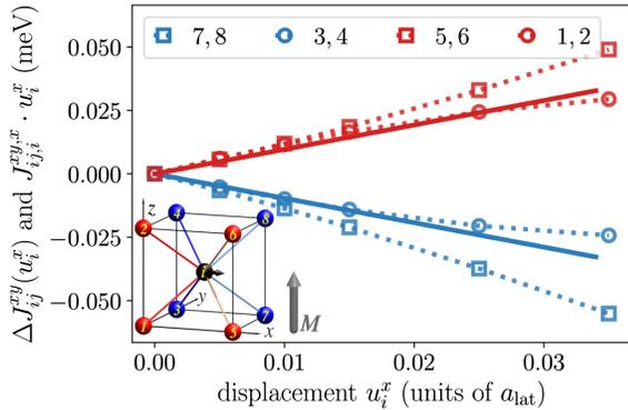
FIG. 1. SLC parameters versus distortion for bcc Fe: Comparison of the products  $\mathcal{J}_{ij,i}^{xy,x} \cdot u_i^x$  (solid lines) with the corresponding SLC terms  $\Delta J_{ij}^{xy}(u_i^x) = J_{ij}^{xy}(u_i^x) - J_{ij}^{xy}(0)$  calculated for a distorted system with the supercell technique (dotted lines) for one atom  $i$  displaced by  $u_i^x$  along the  $x$  axis. The inset shows the labeling of the nearest neighbor atoms used in the figure.
