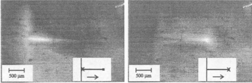
Fig. 2. Flux distribution at 15 K of a laser-patterned rectangle connected with the YBCO film edge by an additional line. Flux distribution during moving the permanent magnet ( $B_{\text{max}}$  at YBCO film distance 300 mT) from the film edge (left) towards the rectangle (right) (The crosses in the insets indicate the position of the magnet in each situation). a) Permanent magnet is located near the film edge. b) Same pattern but 1 sec later when the permanent magnet reached the rectangle.
