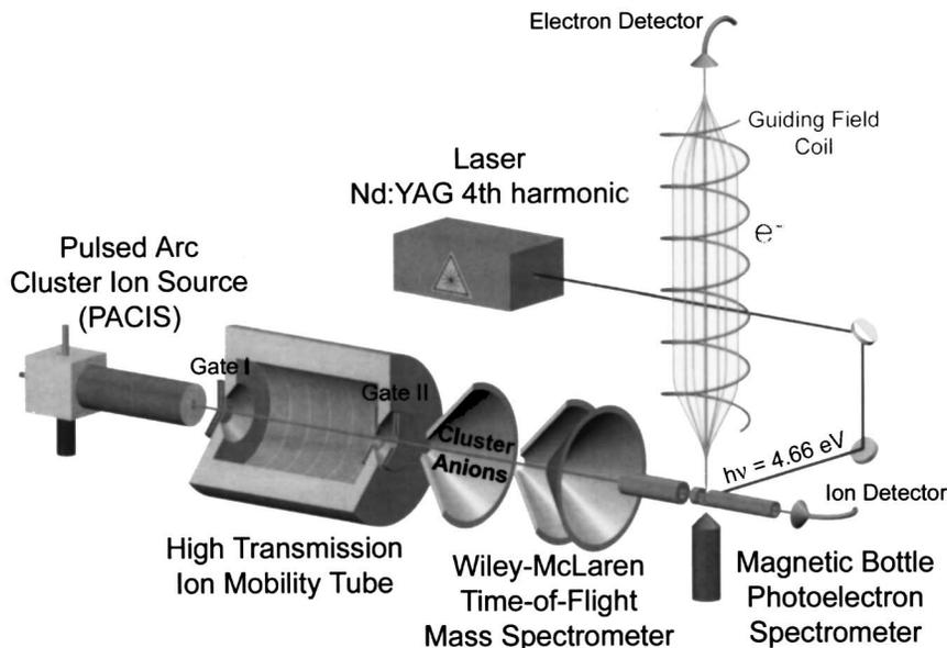
FIG. 1. Schematic diagram of the new IMS/TOF/PES instrument.
