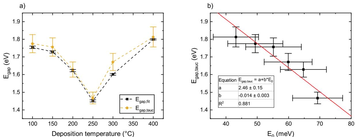
Fig. 4. a) Optical bandgaps  $E_{gap,fit}$  and  $E_{gap,tauc}$  as function of the deposition temperature. Lines as guide for the eye. b) Linear correlation between  $E_{gap,tauc}$  and  $E_0$ . The straight line is a linear fit.
