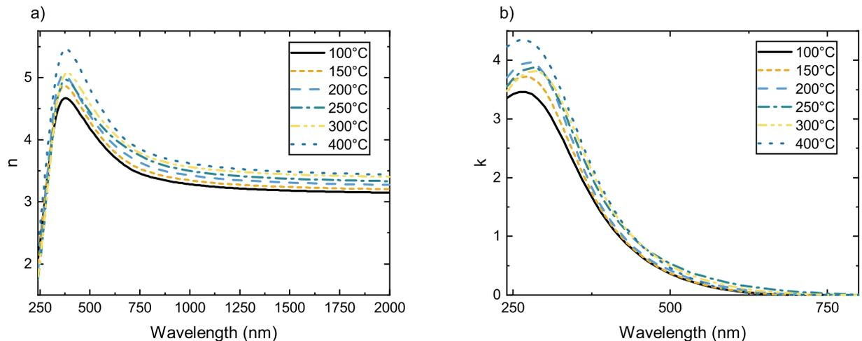
**Fig. 2.** Wavelength dependent optical constants as obtained by the SE fit procedure described in Sec. 2.2 for all deposition temperatures: a) refractive index  $n$  and b) extinction coefficient  $k$ .
