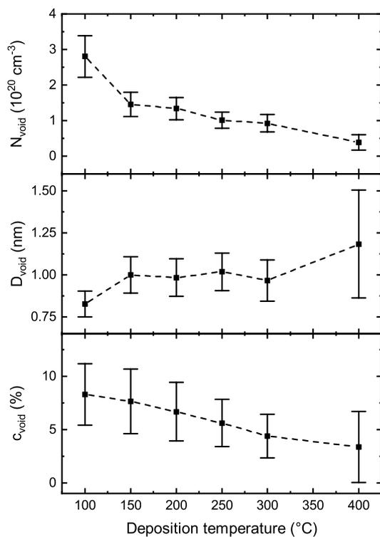
Fig. 3. Microvoid density  $N_{\text{void}}$ , microvoid diameter  $D_{\text{void}}$  and microvoid volume fraction  $c_{\text{void}}$  from Eqs. (8)–(10) as function of the deposition temperature. Lines as guide for the eye.
