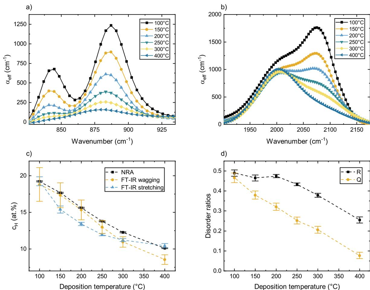
**Fig. 1.** FT-IR measured effective absorption coefficients for a) the bending and b) the stretching absorption band of hydrogen in a-Si:H. c) Hydrogen concentration determined from NRA measurements taken from [13] and from the FT-IR wagging and stretching band (Eq. (4)). d) Microstructure factor  $R$  and ratio  $Q$  according to Eqs. (5)–(6). Lines as guide for the eye.
