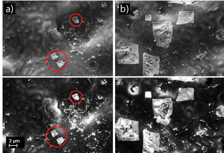
**FIGURE 3.** SEM top view on a laser treated highly doped surface contacted with AgAl paste after contact etching in 5% HF acid. The upper part shows the topography, the lower part the material contrast. The wafer on the left part of the image (a) was fired at a low peak firing temperature T1; the one on the right part of the image (b) was fired using a high peak firing temperature T2.
