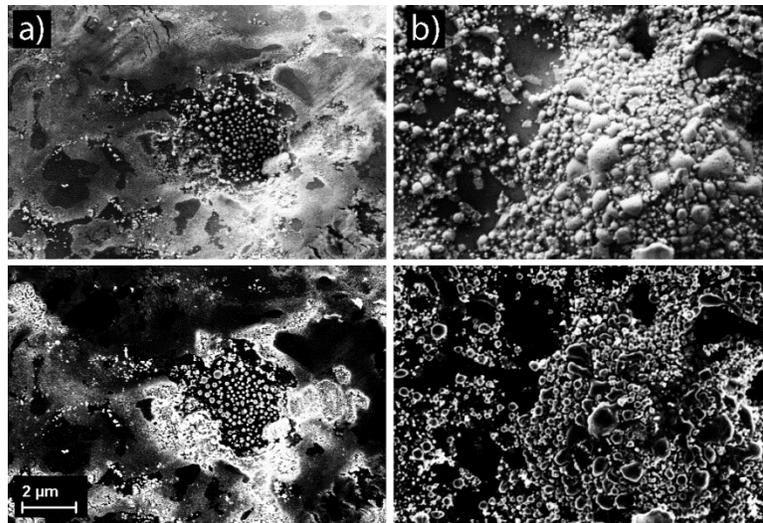
**FIGURE 4.** SEM top view on a laser treated highly doped surface contacted with Ag paste after contact etching in 5% HF acid. The upper part shows the topography, the lower part the material contrast of the same area on the samples for (a) and (b). The sample shown in the SEM image on the left side (a) was fired at a low peak firing temperature T1, the sample shown in the SEM image in the right (b) was fired using a high peak firing temperature T2.
