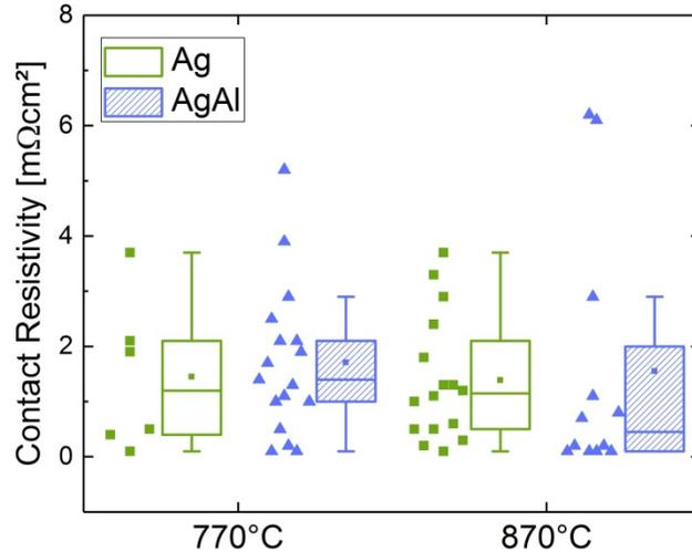
**FIGURE 2.** Measured contact resistivity of the processed TLM structures for the lowest and highest peak firing temperature. Results for the Ag paste are shown by the empty boxes, AgAl paste results are shown by the shaded boxes.
