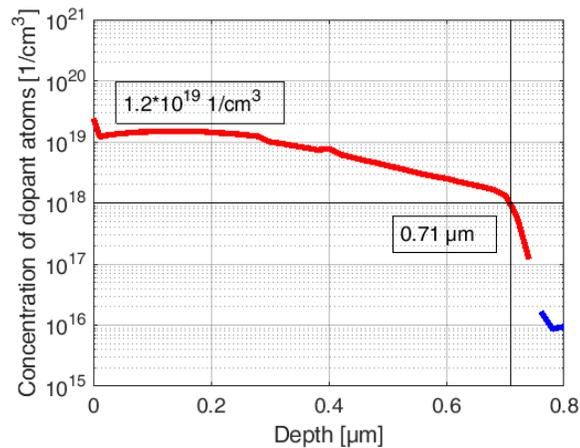
**FIGURE 1.** ECV measurement of the boron emitter structure. The surface concentration is  $1.2 \cdot 10^{19}$  cm<sup>-3</sup>. The profile shows a clear kink at 0.7  $\mu\text{m}$  and the concentration drops rapidly to the base doping.
