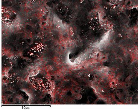
**FIGURE 5.** EDX measurement of a sample contacted with pure Ag paste and fired at T1 peak firing temperature. The red dots show measured Ag on the sample, showing that Ag is distributed all over the wafer surface.
