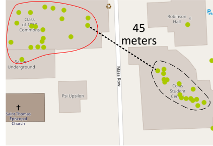
Fig. 5. Assume the minimum distance between the two potential POIs in two buildings is 45 meters, then a stay-point detection or DBSCAN with a distance threshold of 50 meters cannot divide the two clusters. The green color indicates locations belong to one POI resulted from DBSCAN.
