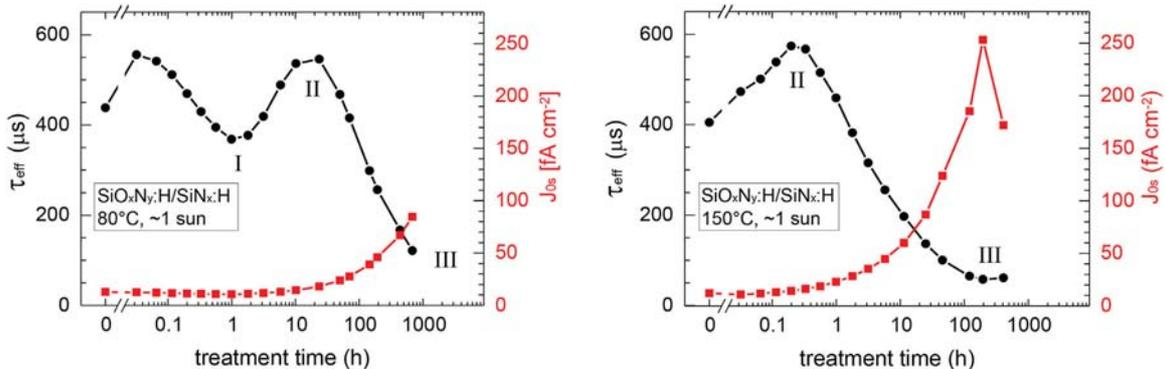
**Figure 2.** Measurement of  $\tau_{\text{eff}}$  ( $\Delta n = 0.1 N_d$ ) and  $J_{0s}$  of Cz-Si samples passivated with a  $\text{SiO}_x\text{N}_y\text{:H}/\text{SiN}_x\text{:H}$  stack during treatment at  $\approx 1$  sun and either 80 °C (left) or 150 °C (right). Part of data taken from Ref. [25].
