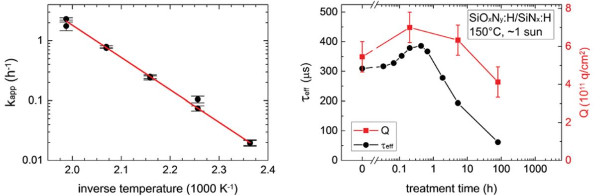
**Figure 6.** (Left) Arrhenius plot of determined degradation rates at different temperatures and  $\Delta n = 0.1 N_d$ . A linear fit yields the apparent activation energy  $E_{\text{app}}$ . (Right) Measurement of  $\tau_{\text{eff}}$  ( $\Delta n = 0.1 N_d$ ) and  $Q$  of a Cz-Si sample passivated with  $\text{SiO}_x\text{N}_y\text{:H/SiN}_x\text{:H}$  during treatment at  $\approx 1$  sun and  $150^\circ\text{C}$ . Part of data taken from Ref. [25].
