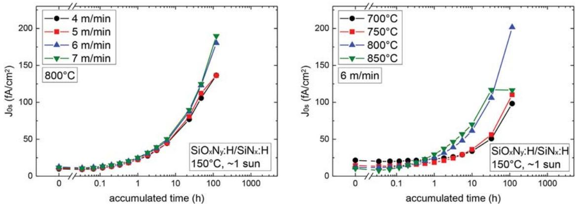
**Figure 4.** Measurement of  $J_{0s}$  of Cz-Si samples passivated with a  $\text{SiO}_x\text{N}_y\text{:H/SiN}_x\text{:H}$  stack during treatment at  $\approx 1$  sun and  $150^\circ\text{C}$  with (left) variation of belt speed and (right) variation of measured peak firing temperature. Part of data taken from Ref. [25].
