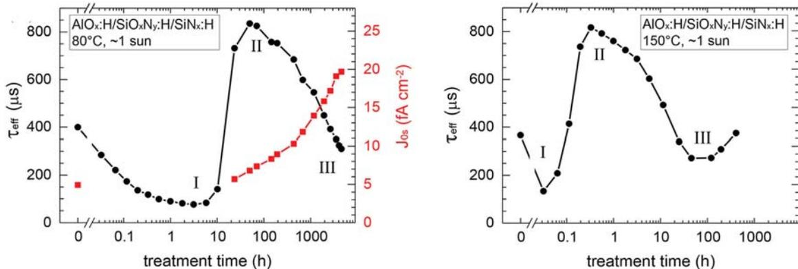
**Figure 1.** Measurement of effective lifetime  $\tau_{\text{eff}}$  ( $\Delta n = 0.1 \cdot N_d$ ) and  $J_{0s}$  of Cz-Si samples passivated with an AlO<sub>x</sub>:H/SiO<sub>x</sub>N<sub>y</sub>:H/SiN<sub>x</sub>:H stack during treatment at ≈1 sun and either 80 °C (left) or 150 °C (right). Part of data taken from Ref. [25].
