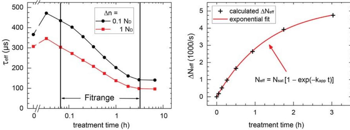
**Figure 5.** (Left) Measurement of  $\tau_{\text{eff}}$  of one of the  $\text{SiO}_x\text{N}_y\text{:H/SiN}_x\text{:H}$  passivated samples used for determining  $E_{\text{app}}$  during treatment at  $\approx 1$  sun and  $210^\circ\text{C}$ . (Right) Values of  $\Delta N_{\text{eff}}$  in a fit range as shown in the left graph. A fit with Equation (2) yields  $k_{\text{app}}$ . Part of data taken from Ref. [25].
