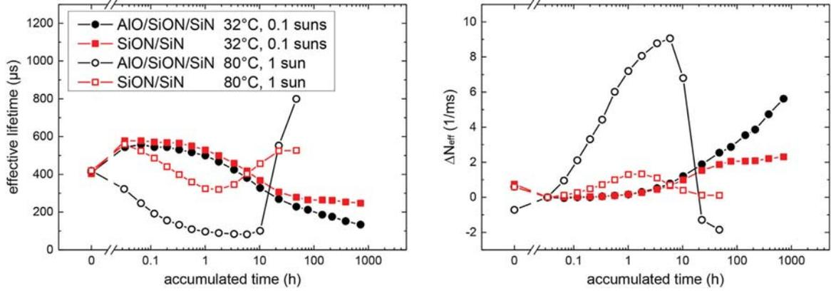
**Figure 3.** Measurement of (left)  $\tau_{\text{eff}}$  ( $\Delta n = 0.1 \cdot N_d$ ) and (right)  $\Delta N_{\text{eff}}$  of differently passivated Cz-Si samples during treatment at either  $\approx 0.1$  suns and  $32^\circ\text{C}$  or  $\approx 1$  sun and  $80^\circ\text{C}$ .
