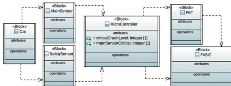
Fig. 3. bdd of the Airbag model
