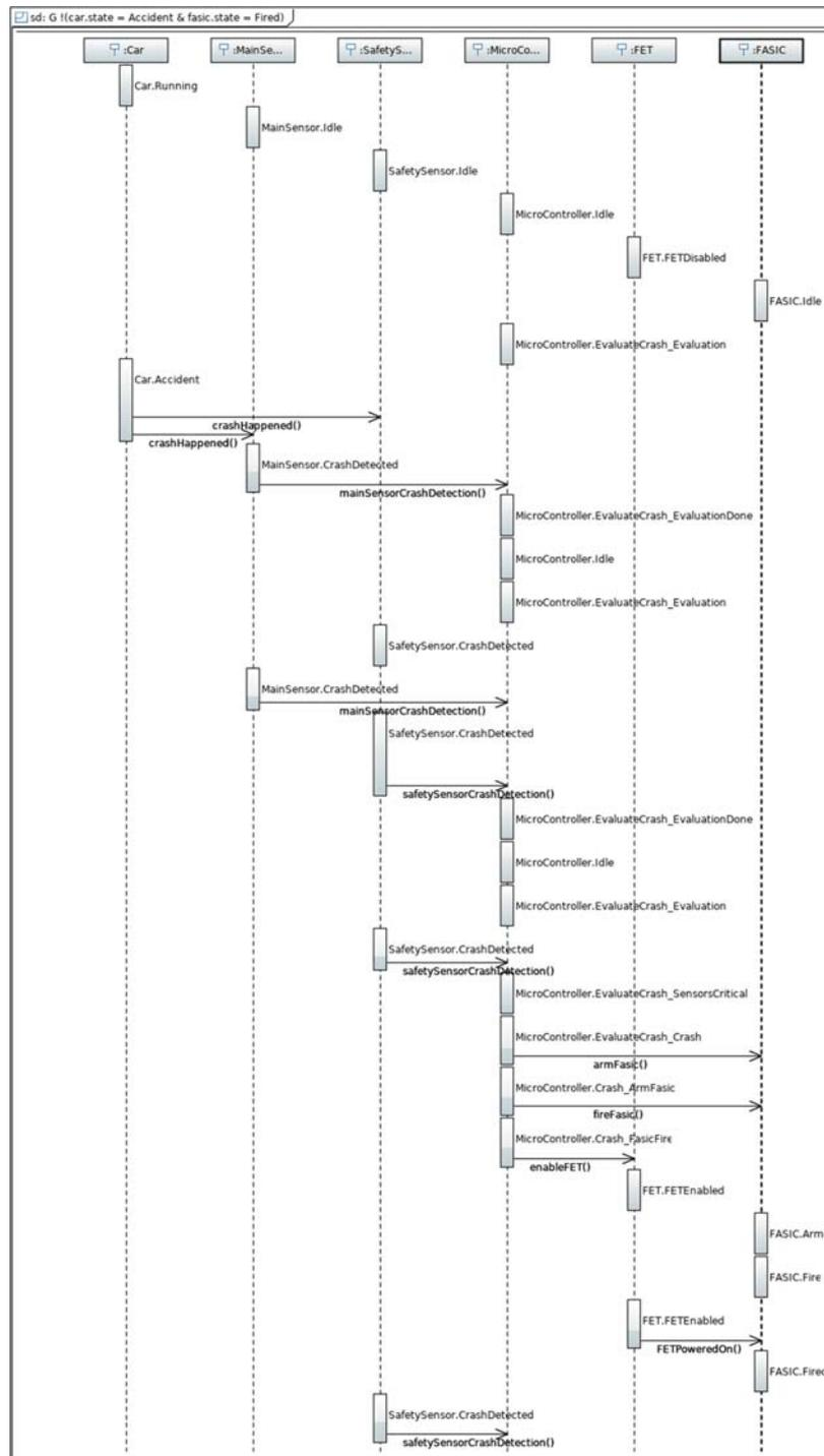
Fig. 4. Sequence diagram depicting the NuSMV2 counterexample, rendered by Papyrus
