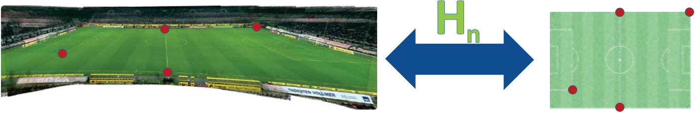
Fig. 3: The chosen points for the transformation of the panoramic (left) into the normalized (right) view must allow referencing distances in both directions of the main axes. Afterwards, a calculated homography H_n enables the transformation of panoramic view into normalized view and vice versa.
