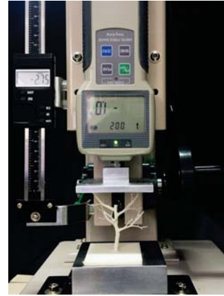
Figure 12: Ground truth evaluation of the printed tree's structural strength by applying a 1N force to a local branch.
