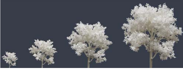
Figure 1: A maple tree ( Acer ) 3D printed using our optimization at several resolutions (left-right). Our algorithm preserved their visual appearance while generating structurally sound tree structures. The tree is 3.7cm, 6.5cm, 10.4cm and 14.4cm in height, respectively.
