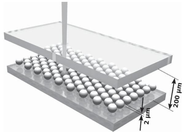
**Fig. 1** A sketch of the sample cell containing the 2D crystal subject to a light-induced substrate (indicated for one particle) and, additionally, pressed down towards the bottom plate by a normal incident laser beam.
