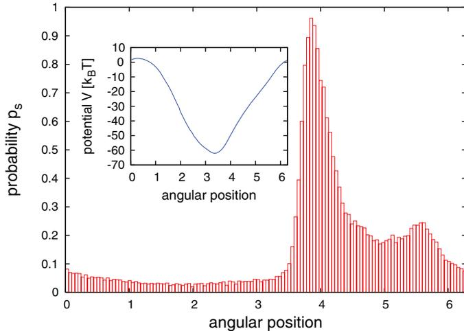
Fig. 1: Stationary probability distribution  $p_s(x)$  for a cosine input signal to the EOM with driving force  $f = 14.2k_B T/\mu\text{m}$ . The inset shows the reconstructed actual potential  $V(x)$  with  $V_0 = 65.6k_B T$ .
