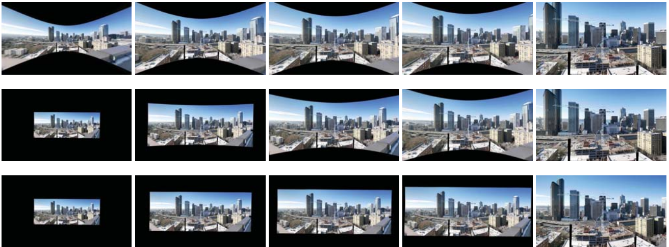
Figure 8: Zooming with perspective projection (top row), cylindrical projection (bottom row), and our adaptive projection (center row). The perspective projection exhibits strong distortion when zoomed out (left column), whereas it produces a natural image when zoomed in (right column). The cylindrical projection produces an undistorted image when zoomed out, but has a less natural appearance when zoomed in. Our adaptive projection combines the best of both worlds. It converges to cylindrical projection for zoomed-out views (left), and to perspective projection for zoom-ins (right).
