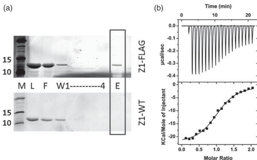
**Fig. 5.** Molecular binding properties of Z1<sup>FLAG</sup>. (a) Pull down assay using anti FLAG M2 affinity gel. The SDS PAGE shows molecular weight markers (M), incubated samples (L), unbound (F: flow through, W1-4: washes) and bound fraction (E: elution); (b) ITC data on the interaction to anti FLAG antibody.
