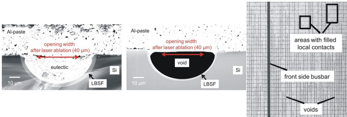
Fig. 1. SEM images of a “filled contact” (left) and a “void” (center). The widening of the contacts during co-firing process is symbolized by the arrow in red, indicating the opening width in the dielectric layer directly after laser ablation. Right: image of the SAM measurement. Thin horizontal lines indicate the front side fingers, running perpendicular to the local rear side contacts. Dark horizontal lines correspond to voids within the local contact area on the rear.
