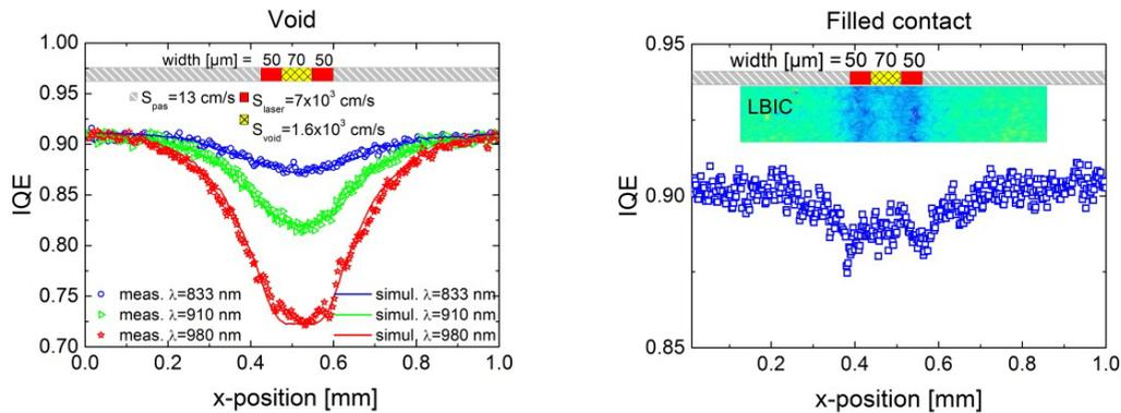
Fig. 3. Left: measured IQE profiles of a void for three laser wavelengths and the corresponding simulated profiles, considering a non-uniform SRV in the void as indicated in the sketch incorporated in the diagram. Right: measured IQE profile of a filled contact, including the corresponding LBIC map ( $\lambda=980$  nm). The measurement fit well to the finding of a non-uniform SRV in the contact area.
