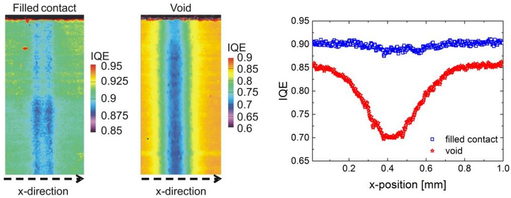
Fig. 2. Left: high resolution IQE mappings of a filled contact and a void ( $\lambda=980$  nm,  $1 \times 2$  mm<sup>2</sup>). The dark lines on top of the images are the front side fingers used to localize the regions of interest. Note the different scaling. Right: line scans in x-direction across the local contacts.
