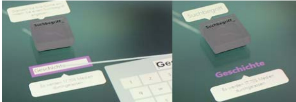
Figure 5. The search term token allows the visitor to specify a search term of interest via touch-typing.
