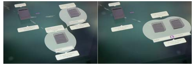
Figure 6. Three filter tokens forming a conjunction of three search terms. The resulting number of items is shown below each token.
