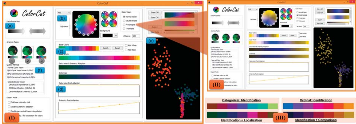
Figure 3: (Ia) The user selects the data type and analysis task combination (① Localization, ② Identification, ③ Comparison) and ColorCAT suggests a colormap design based on the task requirements (see Figure 1). (Ib) The user can select different base colors in the color picker, which allows free adding, removing and rotating knots. (Ic) visualizes the steps of the colormap algorithm for the designer to understand how the base colors are modified to match the analysis task. (Id) Splines allow advanced users to modify intensity and saturation of colormaps. (Ie) The scatterplot allows visual inspection of colormaps and (If) reveals the quality of colormaps. (II) shows ColorCAT simulating red-green blindness. (III) Examples for categorical and ordinal colors.
