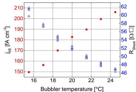
**Figure 5:** The emitter saturation current density (left y-axis) in dependence on the bubbler temperature, measured with QSSPC at an injection density of  $1.5 \cdot 10^{16} \text{ cm}^{-3}$ . The sheet resistance (right y-axis), is measured with 4PP for different bubbler temperatures.
