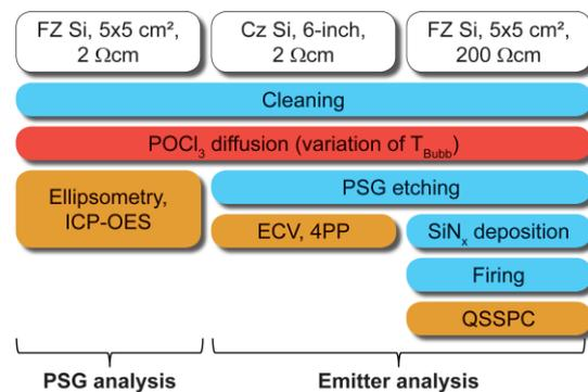
**Figure 1:** Sample preparation for PSG and emitter characterization. For POCl<sub>3</sub> diffusion, several bubbler temperatures (T<sub>Bubb</sub>) were used.
