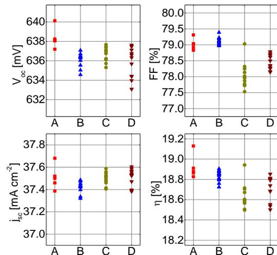
**Figure 6:** IV measurement: Emitter A is our reference with  $\text{POCl}_3\text{-N}_2$  gas flow of  $\Phi_0$  and bubbler temperature of  $20^{\circ}\text{C}$ . Emitter B has a similar sheet resistance, by increasing  $\text{POCl}_3\text{-N}_2$  gas flow and reducing bubbler temperature at the same time. For emitter C  $\text{POCl}_3\text{-N}_2$  gas flow is reduced, while for emitter D bubbler temperature is reduced.
