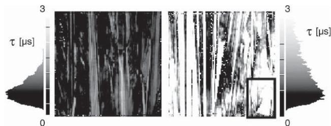
Fig. 1. Typical lifetime mappings of old (left) and new (right) as-grown EFG octagon wafers with passivated surfaces. The marked rectangle is shown in Fig. 3.
