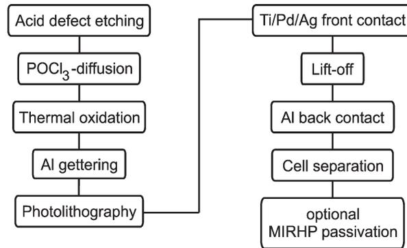
Fig. 4. Processing sequence used for the fabrication of solar cells.
