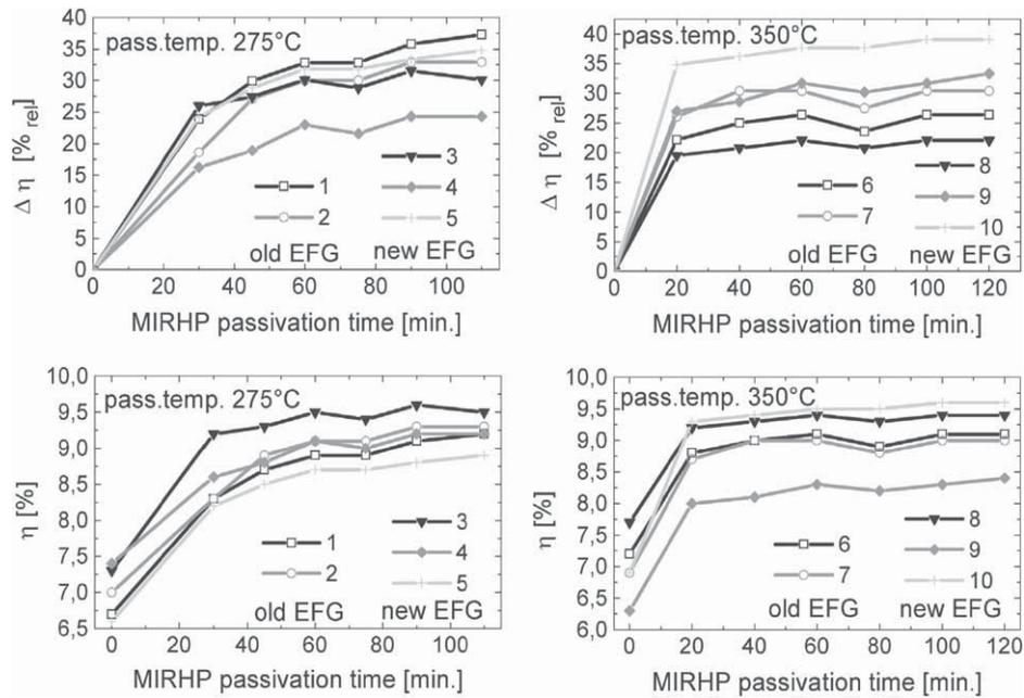
Fig. 8. Relative and absolute efficiency gains in old and new EFG silicon after various hydrogen passivation times at 275°C (left) and 350°C (right).
