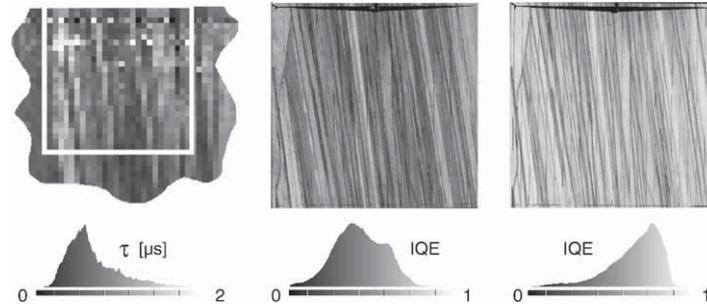
Fig. 5. Clipping of  $\tau$ -measurement of old EFG wafer (left, white square marks — area of interest), IQE (905 nm) of corresponding solar cell (middle) and IQE (905 nm) of the same cell after 110 min of MIRHP passivation at 275°C.
