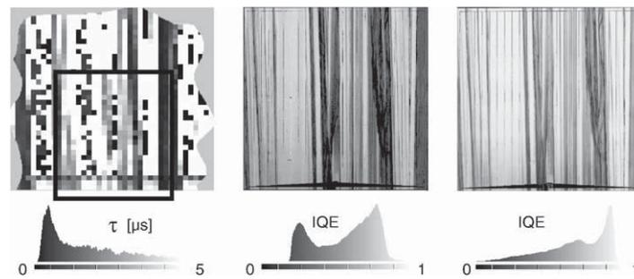
Fig. 6. Clipping of  $\tau$ -measurement of state-of-the-art EFG wafer (left, black square marks—area of interest), IQE (905 nm) of corresponding solar cell (middle) and IQE (905 nm) of the same cell after 110 min of MIRHP passivation at 275°C.
