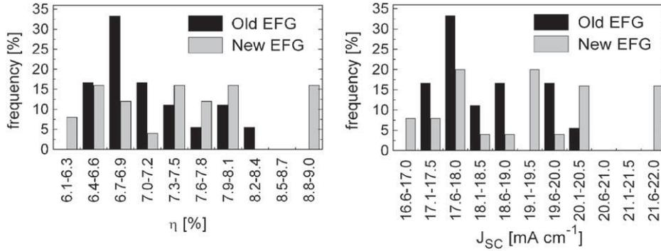
Fig. 7. Frequency distributions of efficiency and short circuit current achieved after cell processing.
