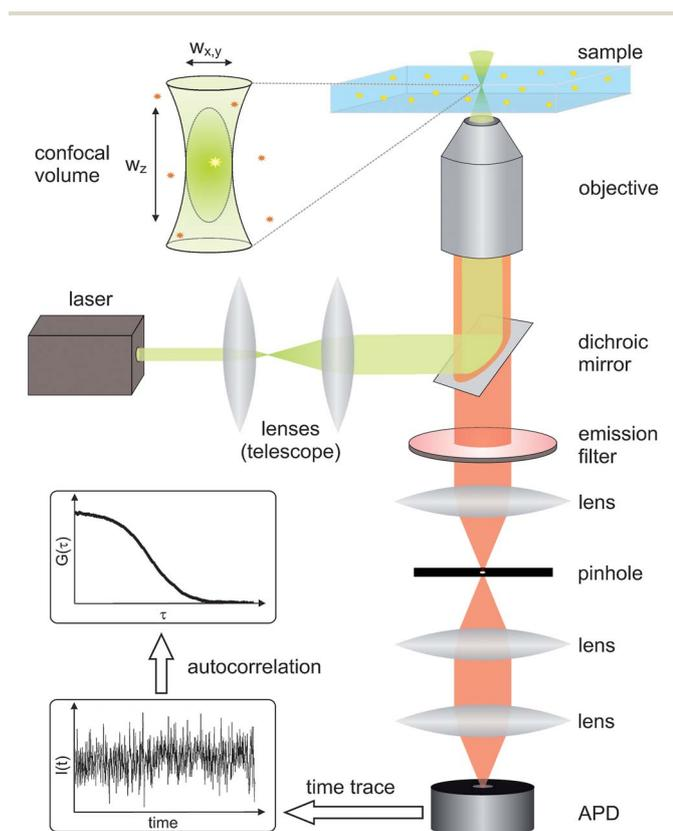
Fig. 1 Typical FCS setup as described in the text.
