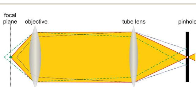
Fig. 2 Effect of the pinhole on the axial resolution of a confocal microscope. Only light originating from the focal plane (red solid line, orange area) can pass the pinhole without loss. Light from other planes (green dotted line and blue dotted line) is mainly blocked.
