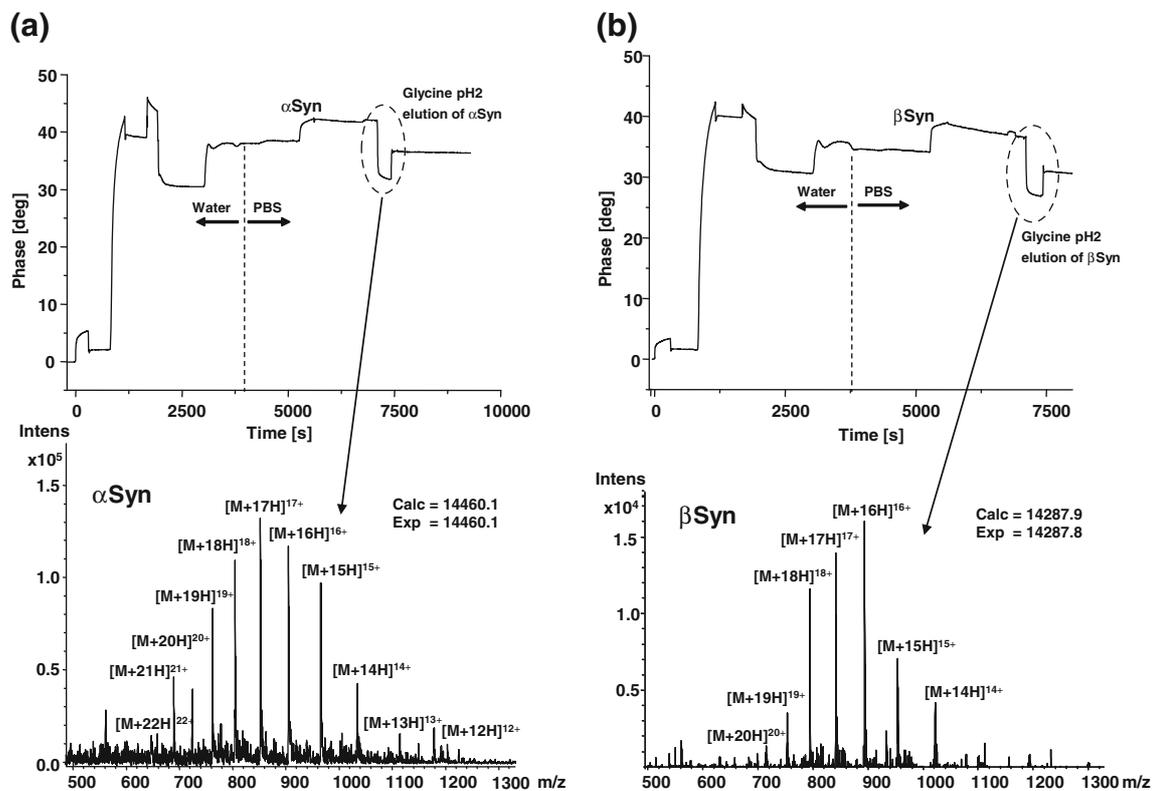
**Figure 4.** Comparison of affinity binding and mass spectrometric identification of  $\alpha\text{Syn}$  and  $\beta\text{Syn}$ . (a) SAW binding curve of  $\alpha\text{Syn}$  to the immobilized anti- $\alpha\text{Syn}$  pC20 antibody and ESI-ion trap mass spectrum of the eluted  $\alpha\text{Syn}$  fraction; (b) SAW binding curve of  $\beta\text{Syn}$  to the anti- $\alpha\text{Syn}$  pC20 antibody and ESI-ion trap mass spectrum of the eluted  $\beta\text{Syn}$  fraction
